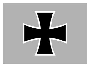
For each complete marking there are 2 masks involved. One is for the White border which is applied first, and the second is for the Black infill.
